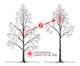
PICTURE 15: Increase of mechanical loading of a tree due to elevation of the centre of gravity may increase the risk of tree failure.
